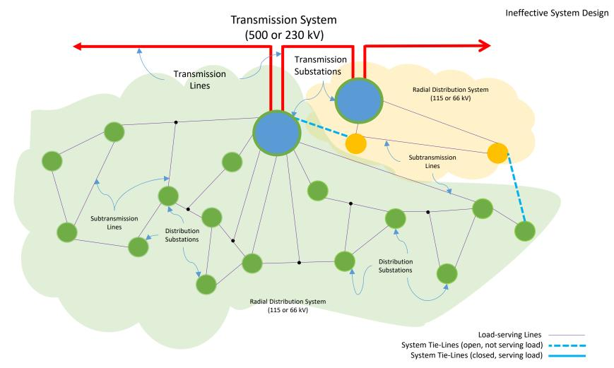
(2) Radial Distribution Systems with *ineffective* system tie-lines *not* located "downstream" at the intersection of the two systems thus not allowing for bidirectional transfer of substations without interfering with the reliable and safe operation of the remaining network following the transfer.
