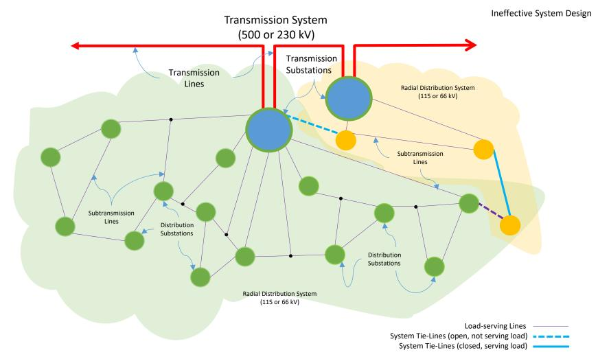
(2) Radial Distribution Systems with *ineffective* system tie-lines *not* located "downstream" at the intersection of the two systems thus limiting bi-directional transfer of substations without interfering with the reliable and safe operation of the remaining network following a transfer.
