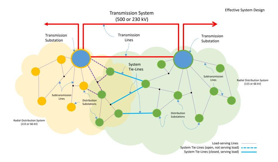
(2) Radial Distribution Systems with <u>effective</u> system tie-lines. Following an incident on the system to the left, the system on the right is able to effectively transfer significant load from the system on the left to provide relief and improving reliability and resiliency.
