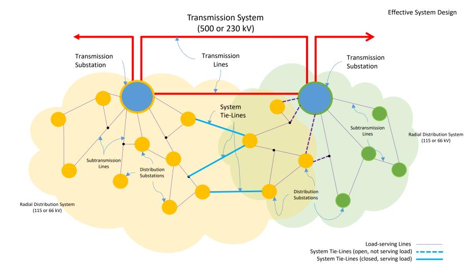
(2) Radial Distribution Systems with <u>effective</u> system tie-lines. Following an incident on the system to the right, the system on the left is able to effectively transfer significant load from the system on the right to provide relief and improving reliability and resiliency.
