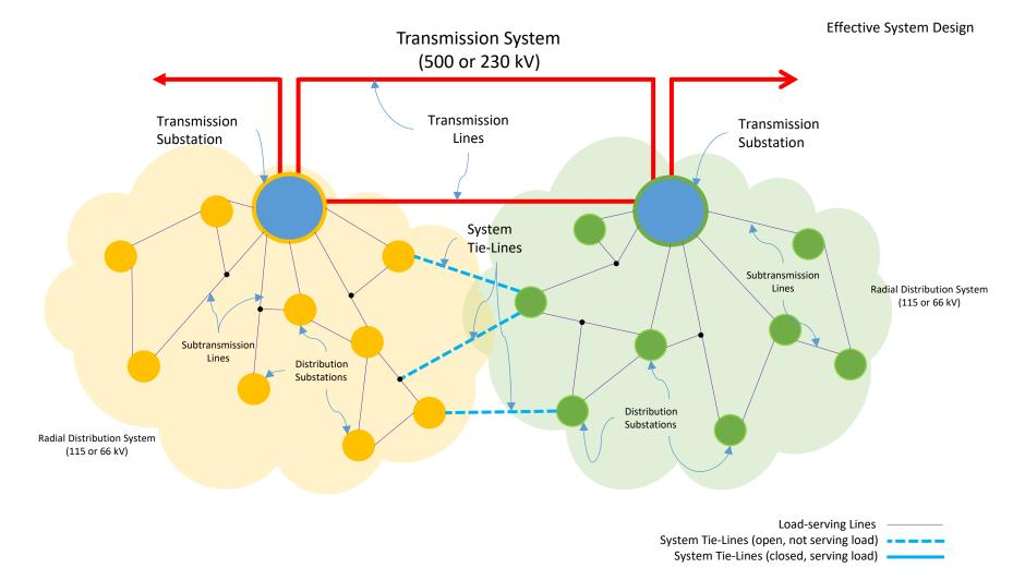
(2) Radial Distribution Systems with <u>effective</u> system tie-lines located "downstream" at the intersection of the two systems thus allowing for bi-directional transfer of substations without interfering with the reliable and safe operation of the remaining network following a transfer.
